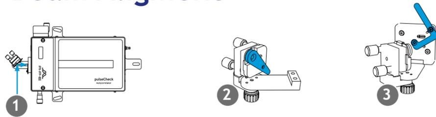
1. Direct the beam at the input mirror.
