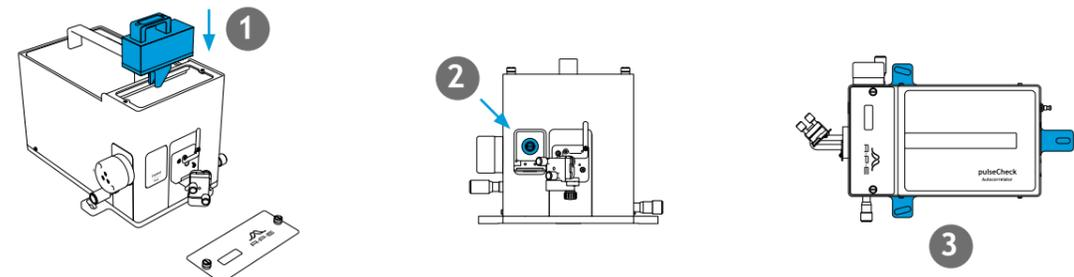
1. Connect the detector cable and mount the detector.
