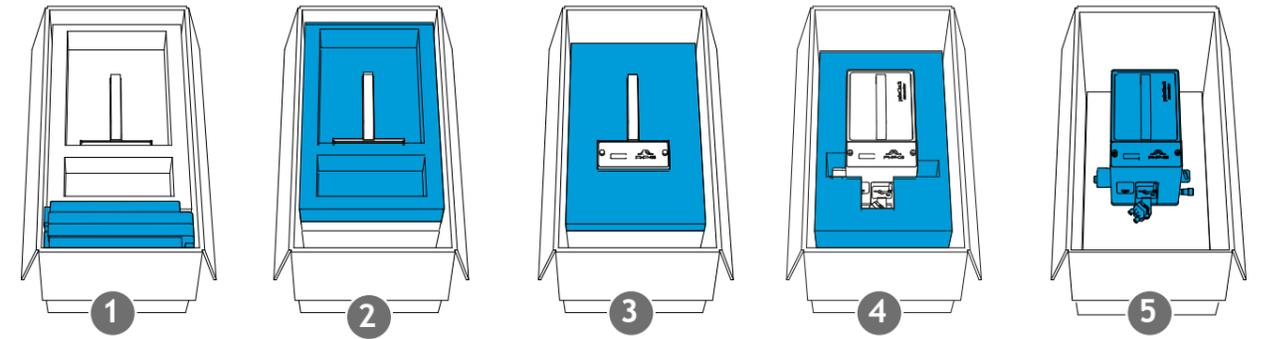
Make sure the box with the pulseCheck had time to reach room temperature to avoid condensation inside the device. Take out the case with pulseCheck accessories. Then remove the foam layers as pictured above.
