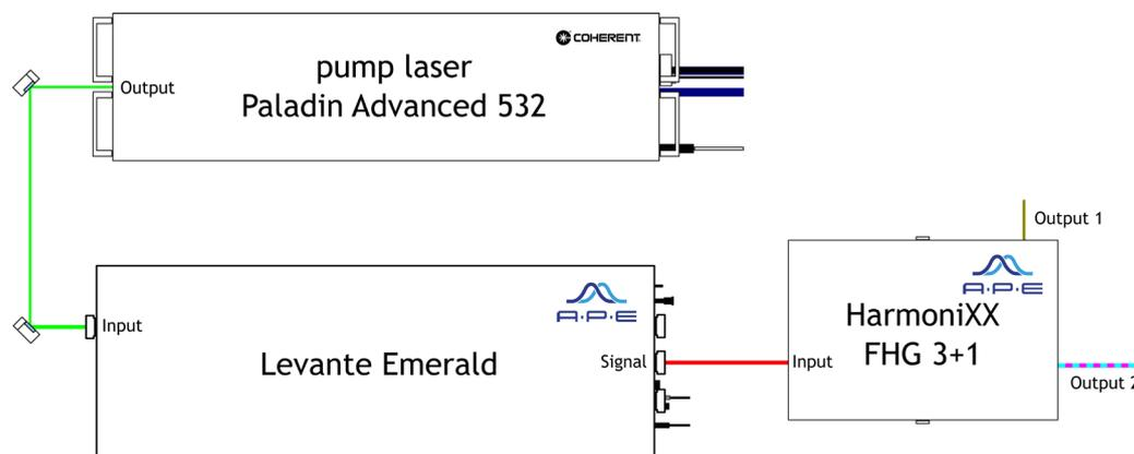
Figure 1: Schematic layout of the UV-light source consisting of a 532 nm pump laser, a sync-pumped OPO and a harmonics generator.
