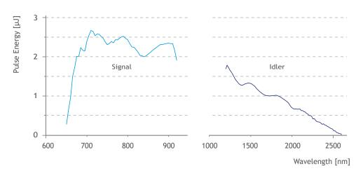
Pulse energy of both signal and idler beam, measured at 40 µJ pump energy.
