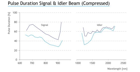
Pulse width of signal and idler beam, both compressed, measured at 40 µJ pump energy.
