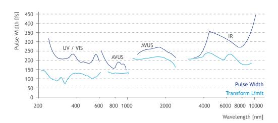
Typical pulse widths (assuming sech<sup>2</sup> pulse shape) and their corresponding transform limits of AVUS including extensions (pumped with 40 µJ pump laser at 1 MHz repetition rate)
