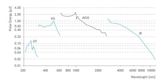
Typical pulse energy vs. wavelength, including UV/VIS and IR extension (pumped with 40  $\mu$ J pump laser at 1 MHz repetition rate)
