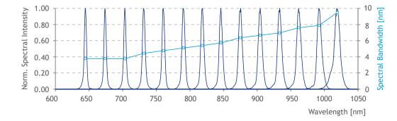
Typical output spectra and corresponding bandwidths (pumped with 40 µJ pump laser at 1 MHz repetition rate)
