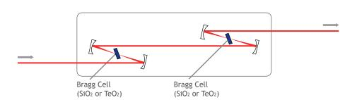
**Dual pulseSelect Parallel:** This variant is designed for simultaneous picking of pulses from two synchronized laser sources. The system is equipped with two synchronized Bragg cells. Independent picking settings are possible for both Bragg cells.
