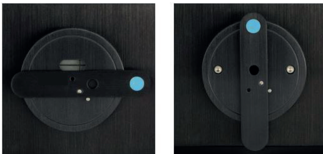
View of alignment window in collinear and non-collinear mode.
